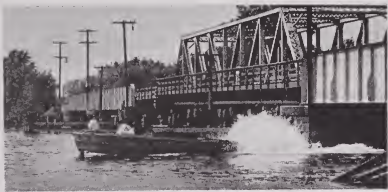
FIGURE 21. Navy plane personnel boat equipped with sine-disk propeller under way at about 13 mph.
